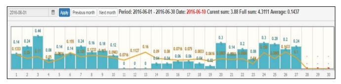
On the appeared schedule it is possible to select desirable day of month and to look on it hourly consumption. At the same time charts in the form of columns show consumption of the chosen meter point, and the crooked line shows average consumption on object.
