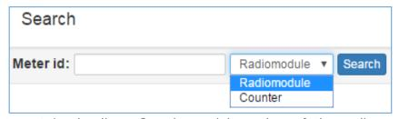
Example: If to set in the line «Search» serial number of the radio module it appears information on this radio module in the form of the table. If to press twice the appeared window, then we get to object in which table there is a radio module.
