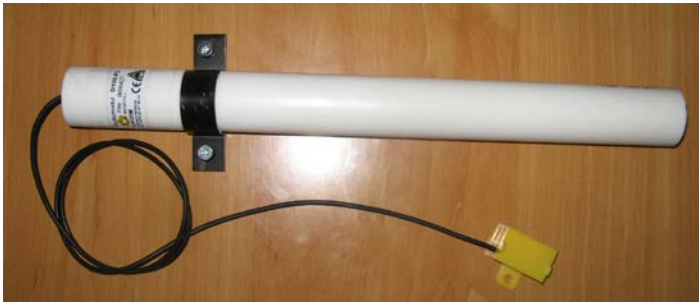
Radiomodule D100-FC-E (diameter of 31 - 33mm, length 320-330mm)
