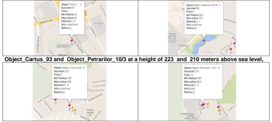
The difference in height of about 186 meters. When one percent error in pressure for every 80 meters, we find that the users are located in the lowland pay for gas by about 2.3% less than the users are located in the higher parts of the city of Chisinau.
